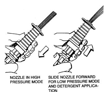
Twisting the nozzle adjusts the spray pattern from a narrow pattern to a fan pattern.
